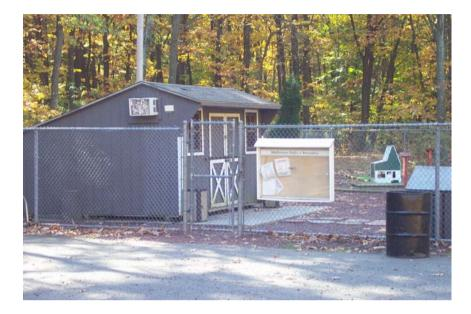
13. There is no access around the golf course because there is no hard ground surface contrary to ANSI section 302.1 and ADAAG section 4.5.1. There is also a transistion more than .25 inches from the entrance to the concrete pad in front of the service window.
